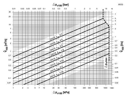
$\Delta p_{max}$  = Maximum permissible differential pressure across the valve (mixing: port A - AB, B - AB), valid for the entire actuating range of the motorized valve
