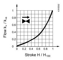
$\begin{array}{lll} 0...30~\% & \rightarrow & linear \\ 30...100~\% & \rightarrow & equal\mbox{-percentage} \\ & & n_{gl} = 3~to~VDI~/~VDE~2173 \end{array}$
