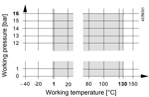
Working pressure and medium temperature staged as per ISO 7005
