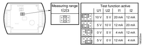
The setting element is located inside the cover. It consists of 6 pins and a shorting plug. It is used for selecting the required temperature measuring range and for activating the test function.
